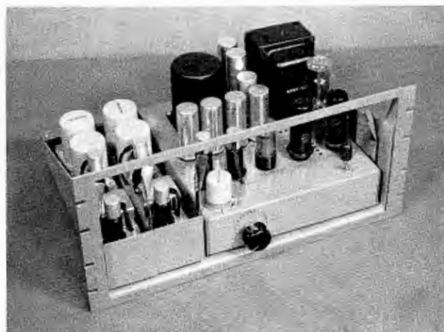
FIG. 20. Two BA-1A Preamplifiers and BA-4A Amplifier on BR-2A Shelf.
