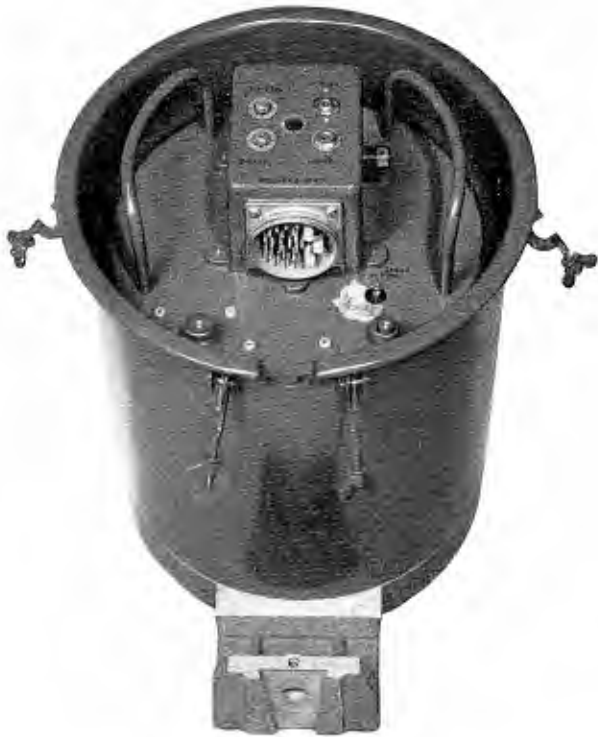
FIG. 15. Receiver case with outer cover removed to show cable connection and metering jacks. Note also the vernier adjustment of "cavity tuning," which is provided on this panel.
