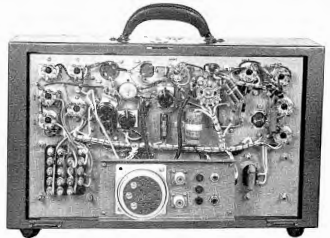
FIG. 14. Rear of the transmitter control unit. Front and rear covers are of the snap-on type, easily removed.
