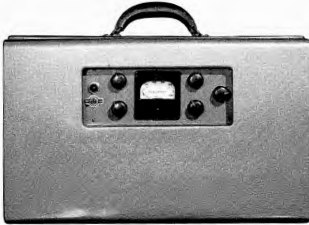
FIG. 12. The transmitter control unit in the convenient carrying case. Both transmitting and receiving equipments are designed to be easily portable.
