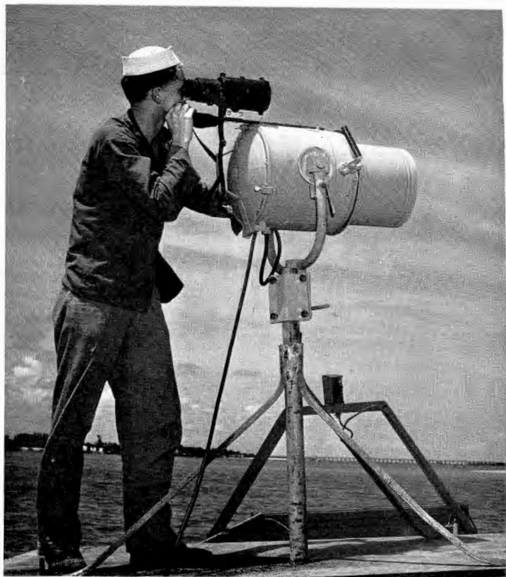
FIG. 2. INFRARED TELESCOPE —This instrument, using a very sensitive image tube in conjunction with an infrared searchlight, is able to pick up (in total darkness) a shoreline a mile away or identify trucks and tanks at 700 feet. The infrared devices shown on this page are only a few of the numerous types developed by RCA engineers.
