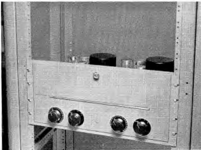
FIG. 10. When mounted on rack, BR-2A Shelf with dial plates and control knobs looks like this.
