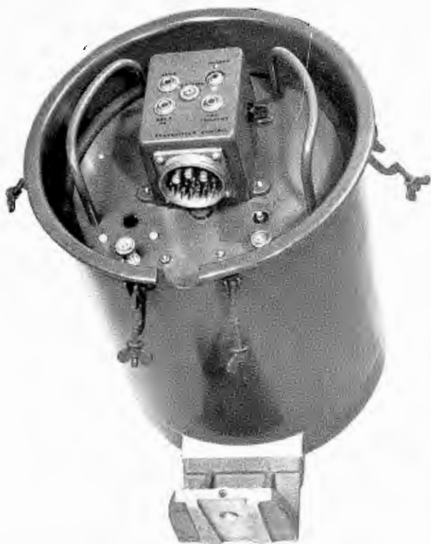
FIG. 9. When the weather-proof back cover is removed, the cable connection (center) and metering jacks are accessible. Cable, which is similar to standard camera cables, allows transmitter control to be located 400 feet away.
