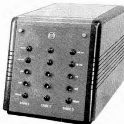
FIG. 8. (Above) Closeup of Sub-control Console. Controls in each vertical row (from top to bottom) are: "On air" light, "In use" light, "On" push-button, "Off" push-button, "Ready" light.
