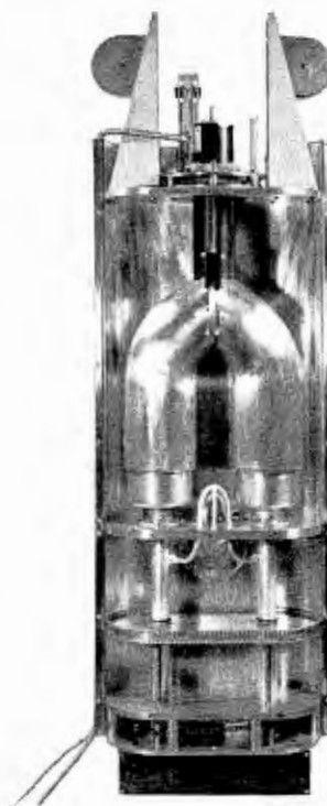
FIG. 11. TANK CIRCUIT—This is an interior view of the one million watt oscillator. The two A-2231 tubes are mounted at the ends of the large "hairpin" in the center. This circuit actually tunes from 560 to 640 megacycles.
