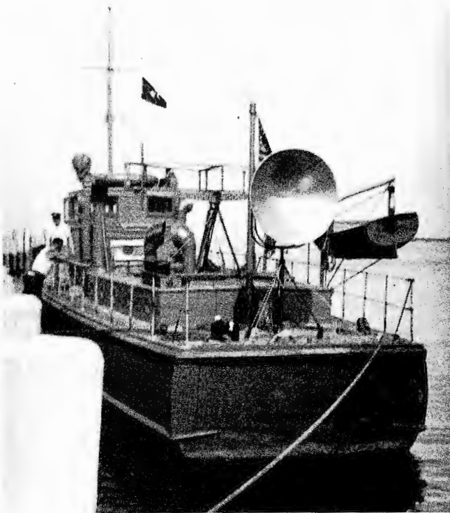
FIG. 5. This view shows the 9 cm. receiver (used with the transmitter shown above) installed on an army boat in New York harbor.
