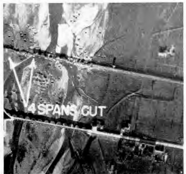
FIG. 13. SHORAN BOMBING —Photo at left shows cluster of bursts from bombs dropped by SHORAN direction on a railroad bridge in Italy. Earlier visual bombing (note old bomb pocks) had failed to destroy this bridge. SHORAN bombing cut four spans as evidenced by photo at right (note lack of shadows for these spans).
