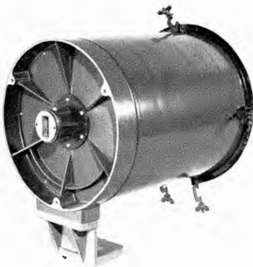
FIG. 4. The transmitter proper is contained in this case. The short transmission line (wave guide in the center) eliminates line losses and impedance matching problems encountered when transmitter and antenna are located at separate points.
