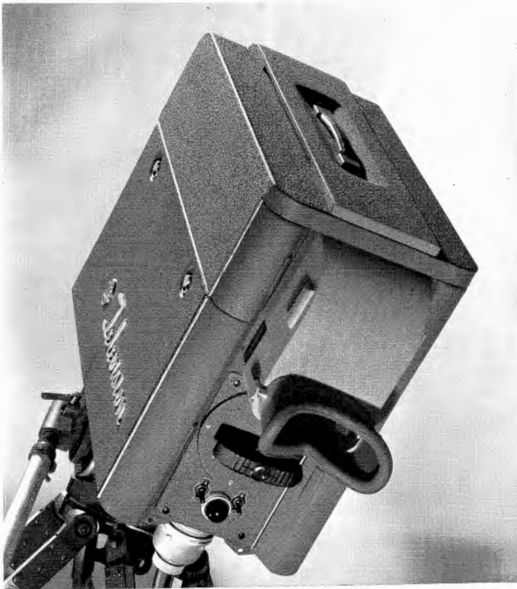
(Left) Side view of the RCA Type TK-30A Field Camera which uses the Image Orthicon tube.
