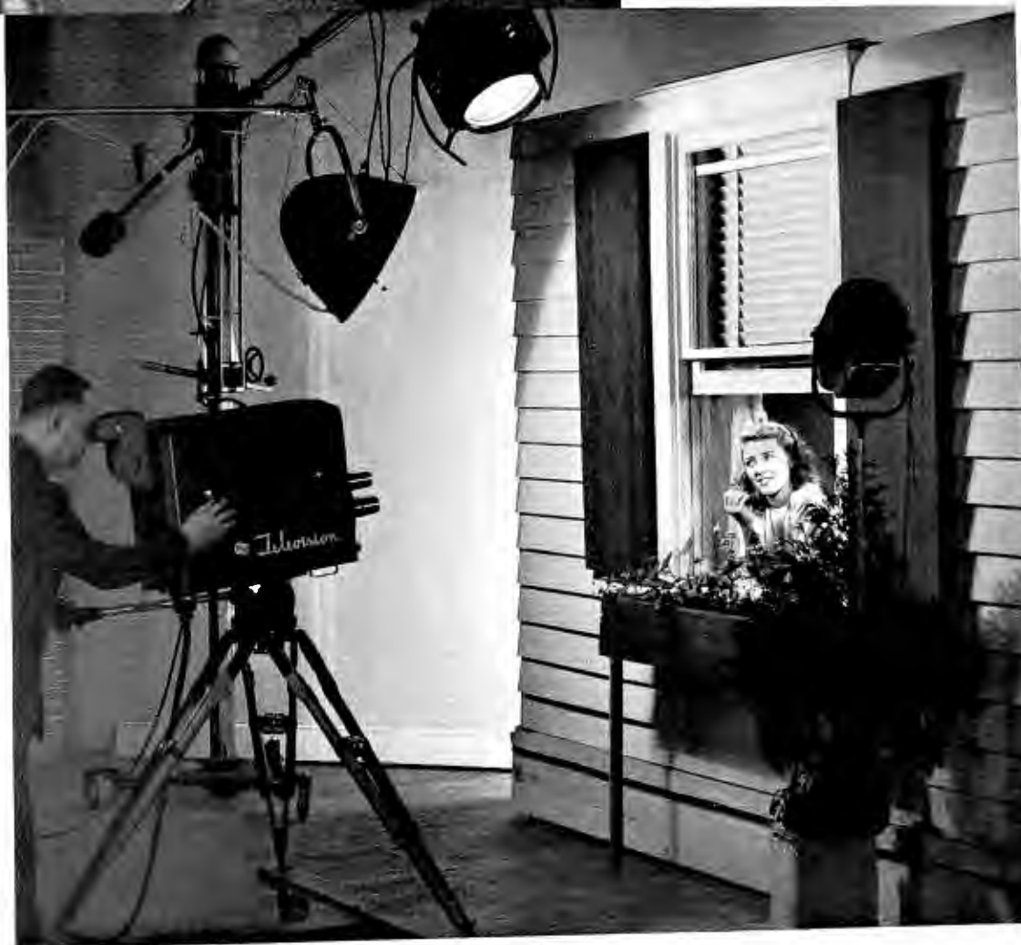
CAN BE USED IN THE STUDIO —While the TK-30A Camera was especially designed for field use, it is believed that it will also be satisfactory for most types of studio programs. For such use the tripod may be mounted on a dolly (as shown at right) so that it can be moved around more easily. Or it may be removed from the tripod and mounted on a more elaborate type of pedestal.
