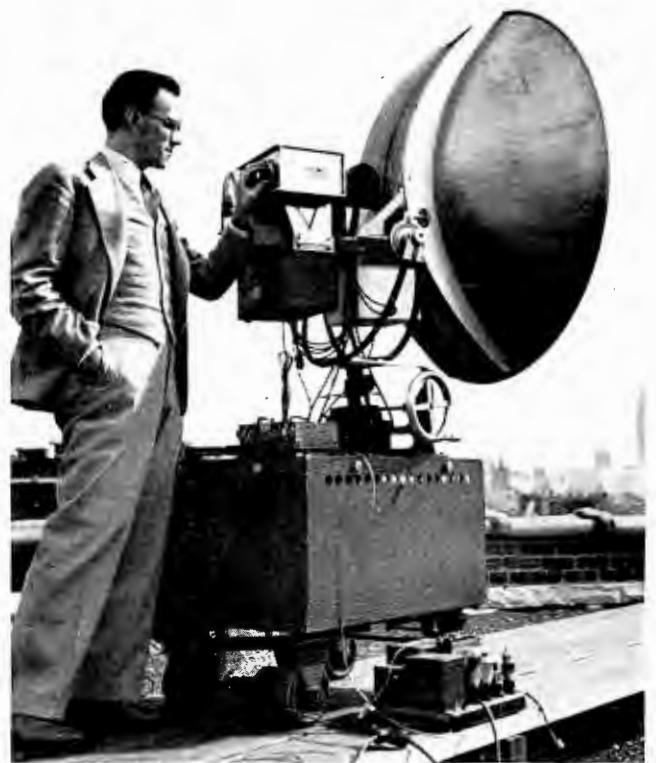
FIG. 6. This view shows Dr. Linder with a 9 cm. pulse transmitter located on the roof of an RCA building in Camden in 1936.
