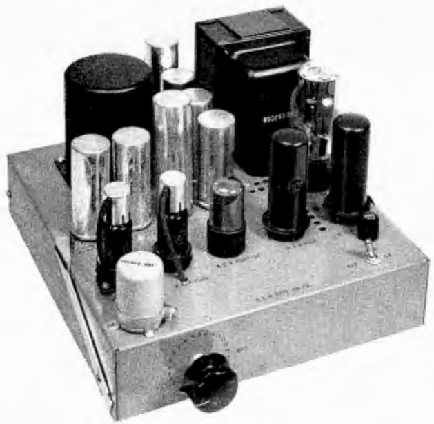
FIG. 15. Type BA-4A Monitoring Amplifier is a high-fidelity, 12-watt amplifier for driving control room and audition speakers.
