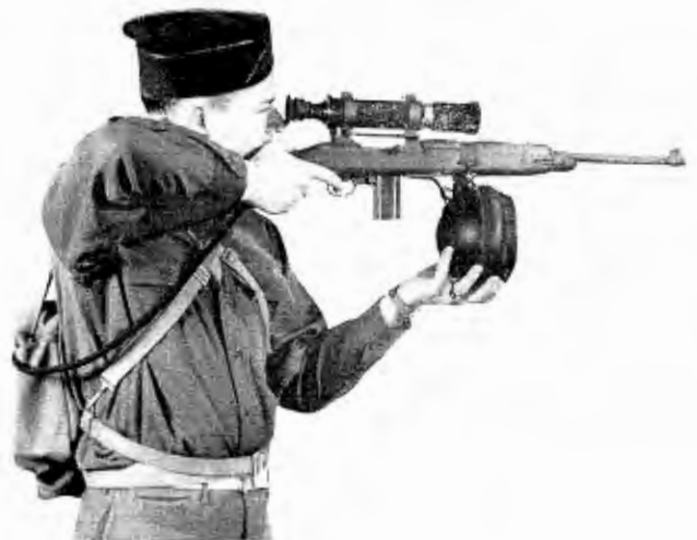
FIG. 3. SNIPERSCOPE —An infrared spotlight and image tube sight mounted on a carbine made it possible for U. S. infantrymen to identify and kill an enemy at 150 feet in total darkness. This weapon alone accounted for 30% of Jap casualties on Okinawa. This is the prototype which was developed by RCA.
