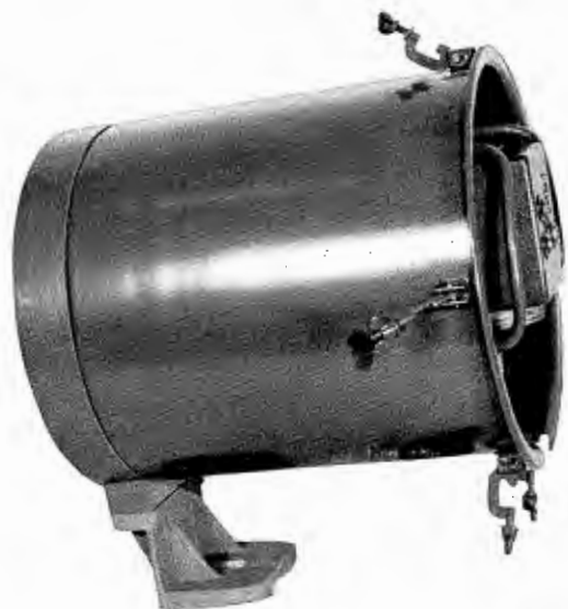
FIG. 5. For maintenance or replacement the transmitter chassis can be removed from the case by loosening three thumb nuts. No connections need be removed.
