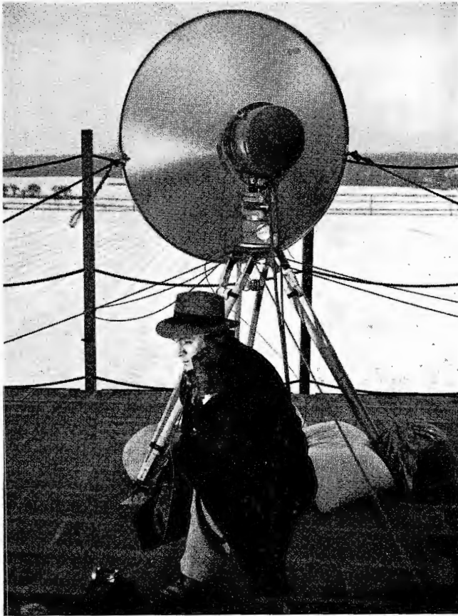
FIG. 3. Where used for remote pickup (at football games, prizefights, etc.) the antenna, parabolic reflector, and attached transmitter will usually be placed in a temporary position on the roof of the stadium or other high point. The transmitter control unit may be mounted in a more convenient position (for instance, with the camera control units) and may be as much as 400 feet away.
